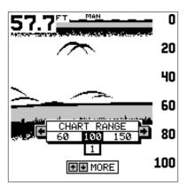
150, 200, 300, 500, 800, and 1000 feet. After the desired range is displayed, press the EXIT key to erase the range menu.
